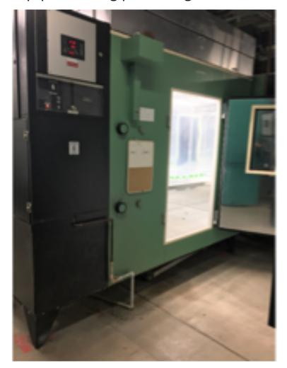
Figure 1, left: A growth chamber used for controlled environment plant science research.
