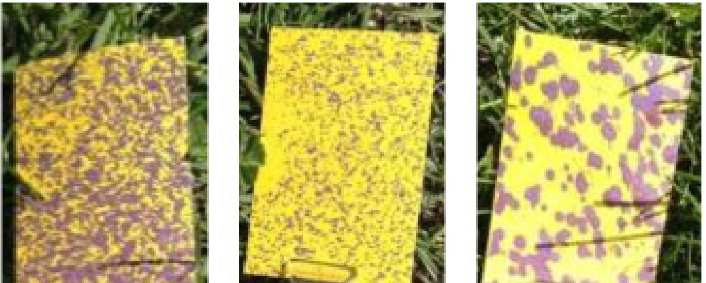
Image 1: Water sensitive paper showing the spray droplet distribution from three different nozzles
