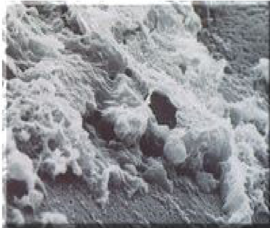
Organic acid coatings responsible for water repellency on a sand particle. Photo Dr. Keith Karnok, University of Georgia DR.
