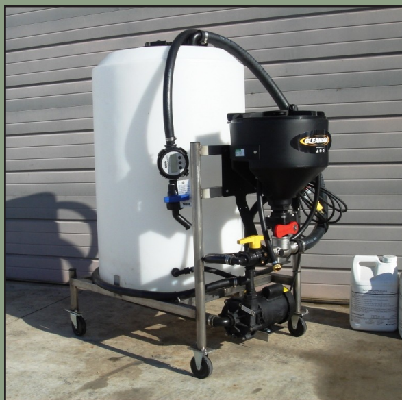
Chemical Pre-mix Station
