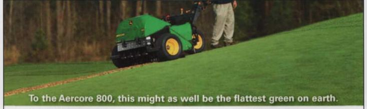
It's all the same to us. Because whether a green has a severe slope, rolls a little bit, or has no roll at all, our Aercore" 800 Walk-Behind Aerator can produce an even depth of coring on all of them. Unlike some walk-behind aerators that position the conng heads behind the wheels, the Aercore 800 has its coring head between the wheels. This allows the coring head to stay at a consistent level to the ground. And produces the same length of plug, again and again.
