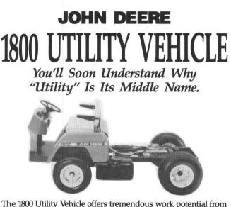
The 1800 Utility Vehicle offers tremendous work potential from one basic machine. Foot-controlled hydrostatic drive gives you an immediate advantage. Teamed with the gutsy, liquid-cooled 18-hp engine, this drive system delivers infinite speed control for precise operation. Great for jobs ranging from spraying to spreading to hauling. Other advantages include power steering, cruise control, wide stance and simple access.
