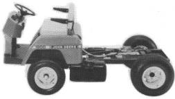
The 1800 Utility Vehicle offers tremendous work potential from one basic machine. Foot-controlled hydrostatic drive gives you an immediate advantage. Teamed with the gutsy, liquid-cooled 18-hp engine, this drive system delivers infinite speed control for precise operation. Great for jobs ranging from spraying to spreading to hauling. Other advantages include power steering, cruise control, wide stance and simple access.
