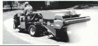
Mount the TD 1500 on your Turf-Truckster® or the TD 1000 on your Jr. Turf-Truckster for high performance, efficient top dressing. The textured surface design of the TD 1500 endless conveyor belt distributes materials evenly for maximum effect.
