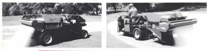
Mount the TD 1500 on your Turf-Truckster<sup>®</sup> or the TD 1000 on your Jr. Turf-Truckster for high performance, efficient top dressing. The textured surface design of the TD 1500 endless conveyor belt distributes materials evenly for maximum effect.
