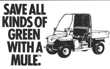
Introducing the Kawasaki Mule. A new utility vehicle engineered to make turf care easier and quicker. A mighty 454cc, 18 hp. liquid-cooled engine delivers torque and power smoothly and quietly. For nimble handling, there's rack and pinion steering and independent front and rear
