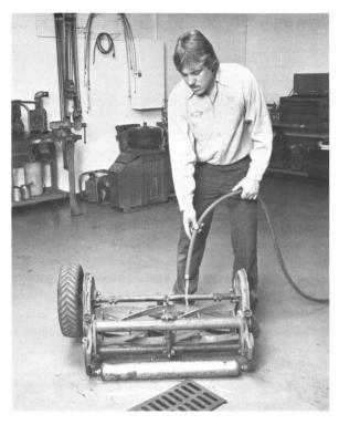
After the blade assembly spins quietly and final adjustments have been made, flush the reel sharpening from the unit. With safe, biodegradable compounds, the rinse water can enter sewage and drainage systems without fear of pollution.
