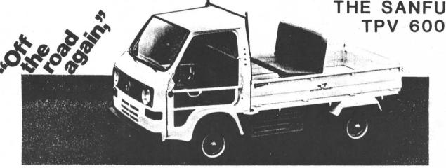
With the Sanfu TPV 600, the work horse for hauling people and cargo off-road. Its 27 h.p., overhead cam, gasoline engine and four-speed, syncromesh transmission give the Sanfu powerplus.
