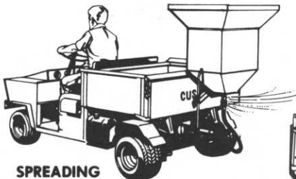
SPREADING Spread up to 40' swath.
