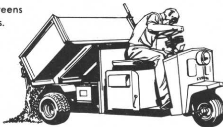
DUMPING/HAULING 1000 lb. payloads. Manual and hydraulic dumping.
