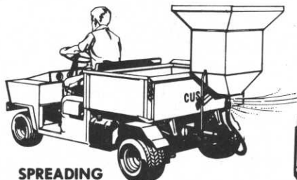
SPREADING Spread up to 40' swath.
