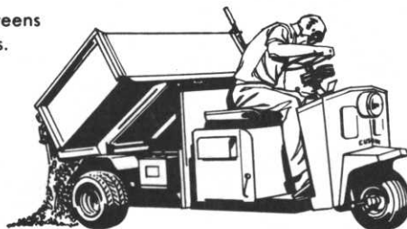
DUMPING/HAULING 1000 lb. payloads. Manual and hydraulic dumpings.
