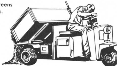
DUMPING/HAULING 1000 lb. payloads. Manual and hydraulic dumping.
