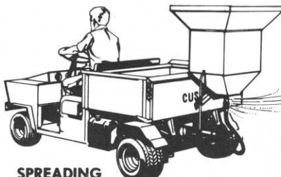
SPREADING Spread up to 40' swath.
