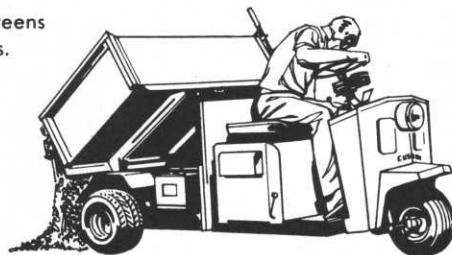
DUMPING/HAULING 1000 lb. payloads. Manual and hydraulic dumpina.
