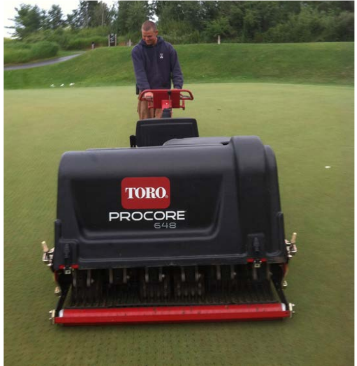
Luke needle tining greens a putting green at Blackwolf Run during his internship.
