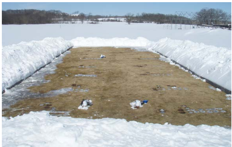
Figure 1. The inner portion of the winter degradation research plot was kept free of snow by shoveling the snow onto the outside of the plot following every snowfall. Several weather stations can be seen on the non-snow covered plots.
