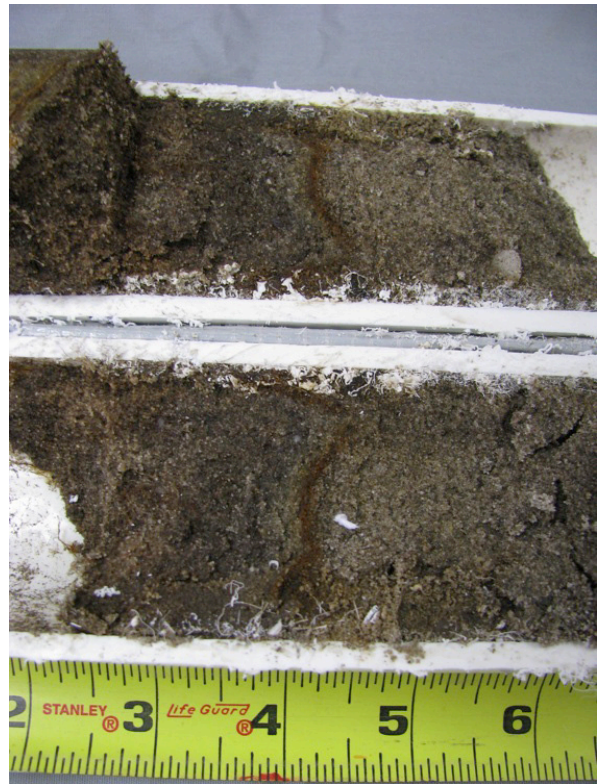
Figure 2. An iron layer is beginning to form at about four inches down because of a textural discontinuity where fine topdressing sand sits on top of the original root zone mix. (Image: Obear)
