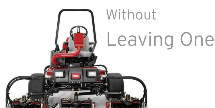
The new Toro® Reelmaster® 3550-D floats effortlessly over contours in fairways and green surrounds. Featuring a productive 82" cutting width, turf friendly tires, a Tier 4 compliant engine, the superior traction of a Series/Parallel 3-wheel drive system, and a weight of less than 2,000 pounds\*, the Reelmaster® 3550-D is the new lightweight fairway champion.
