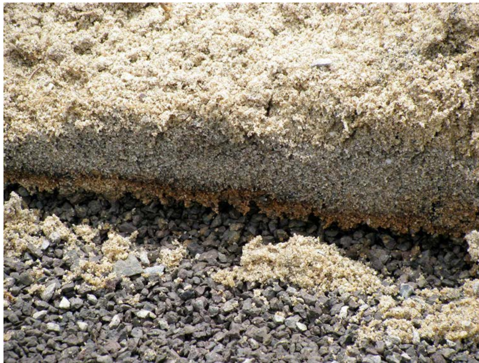
Figure 3. An impermeable iron layer at the sand/gravel interface in a USGA putting green. Photo: Glen Obear
