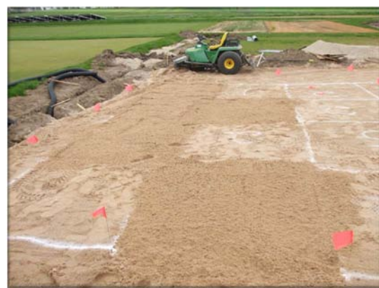
Figure 1. Various amounts of monopotassium phosphate fertilizer were incorporated into 32 plots during construction of the putting green with a rototiller. This method resulted in a broad range of Mehlich-3 soil test phosphorus levels and turfgrass deficiency symptoms.
