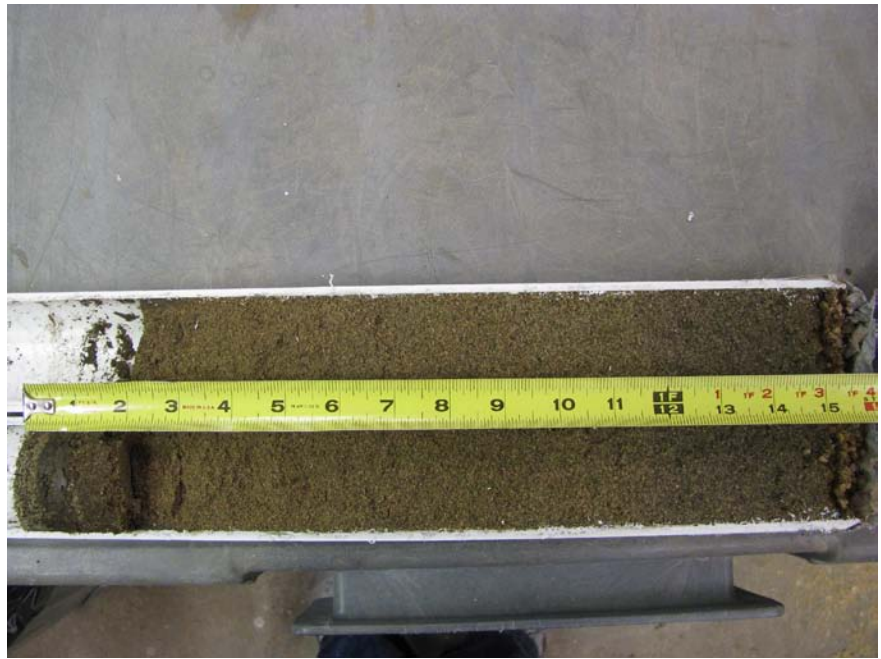
Figure 3. Full putting green profile sample. Note the iron layering at 15" depth.
