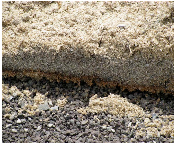
Figure 2. Iron oxide layer observed at the sand/gravel interface (12" depth) of a putting green.
