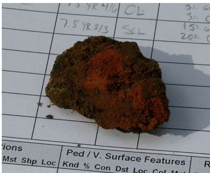
Figure 1. Redoximorphic features in a natural soil. Red color is oxidized iron (i.e., rust).
