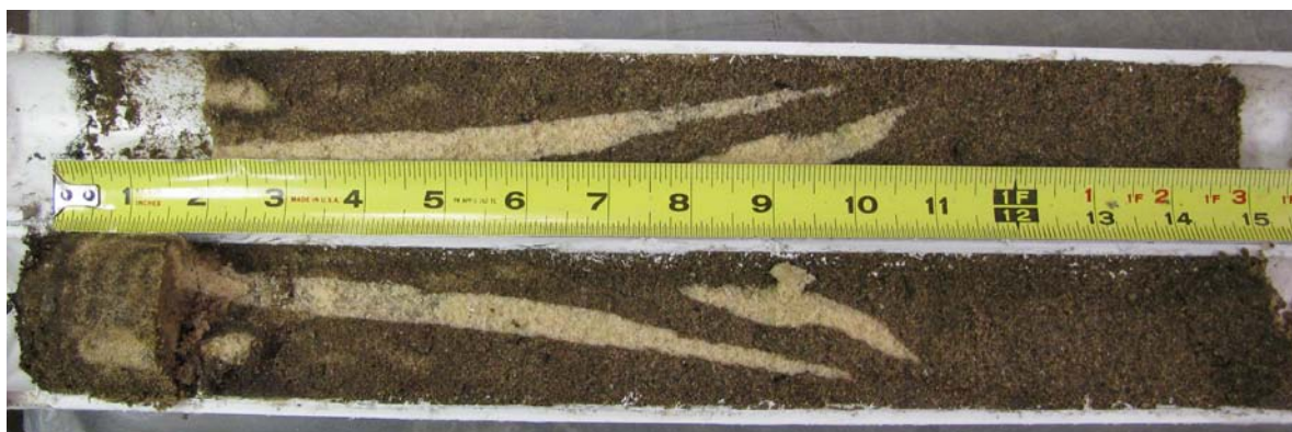
Figure 4. Full profile sample of sand putting green. Sand channels are from deep tine aeration.
