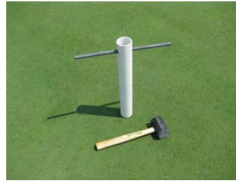
Figure 1. 20" PVC pipe with sharp edge on bottom and hole drilled in top for handle
