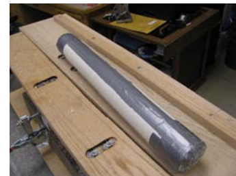
Figure 1. 20" PVC pipe with sharp edge on bottom and hole drilled in top for handle
