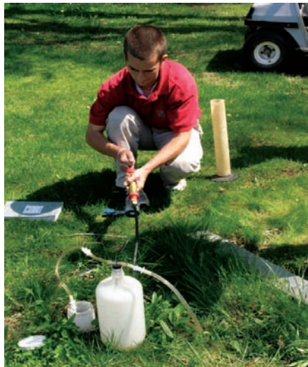
Fig. 2. Graduate student Jake Schneider pumps a lysimeter sample from below-ground of a buffer strip plot at Wisconsin River Golf Course, Stevens Point, WI.
