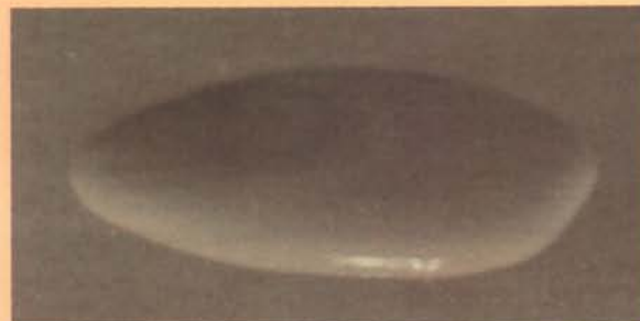
Figure 3. When a surfactant is added to water, the cohesive forces decrease and the water droplet spreads out along the wax surface. The amount of water in this picture is exactly the same as in Figure 2.
