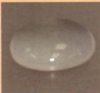
Figure 2. A drop of water sitting on wax paper forms a droplet because the water's cohesive forces are larger than the adhesive forces between the wax and the water.
