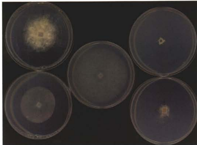
Figure 1. This is an example of the process used for rating the level of resistance to DMI fungicides. The plate in the middle is growing on media not amended with fungicide, while the outside four plates are growing on media amended with propiconazole. The lack of growth of the two on the right suggest it is sensitive to the fungicide, while the significant growth of the two on the left suggest a certain level of resistance to propiconazole.
