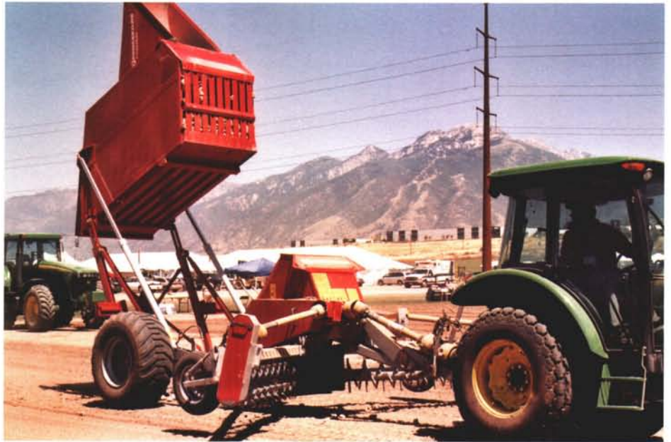
This Kongskilde rock picker was also demonstrated at Biogress, and is the same model we used to prepare the new fields at O.J. Noer.
