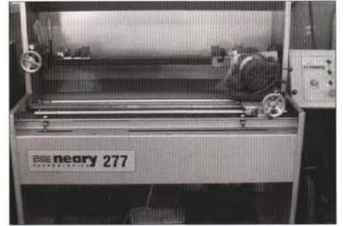
Neary grinders for sharpening reels and bed knives
