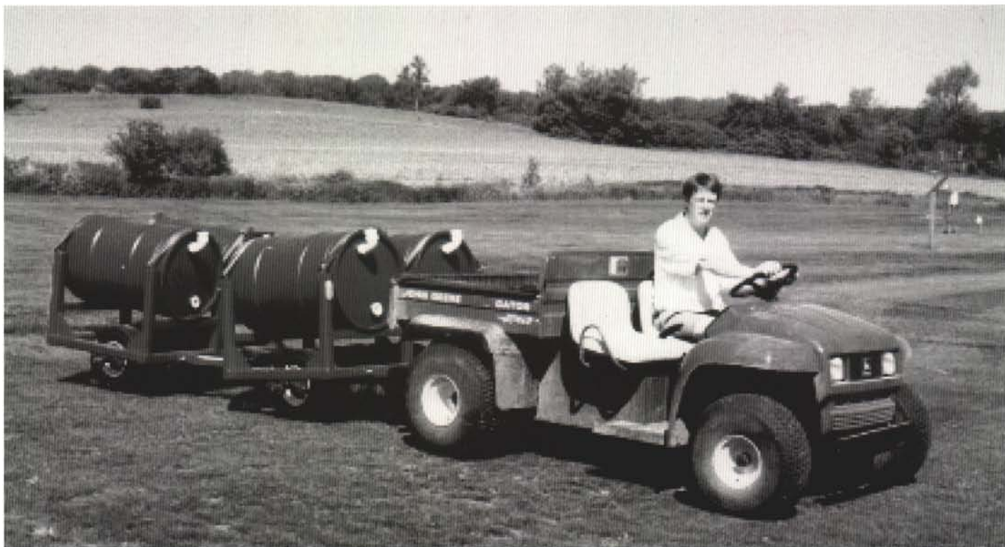
Golf cart traffic simulator for testing traffic tolerance of fine fescue cultivars.
