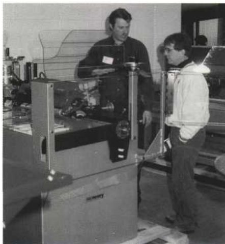
Brent Ackley (L), of Neary Technologies, shows Jeff Kingsley, golf course superintendent of New Berlin Hills G.C., the features of a reel and bed knife grinder.
