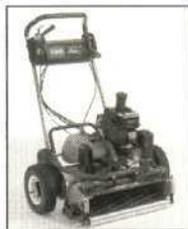
The key to the innovative Flex 21 is a flexible cutting unit. The unit not only flexes from side to side around the bedknife, but also forward and backward around the reel centerline, providing a crisp, clean cut. This is a must for cutting undulating greens and the new Ultra Dwarf grasses.
