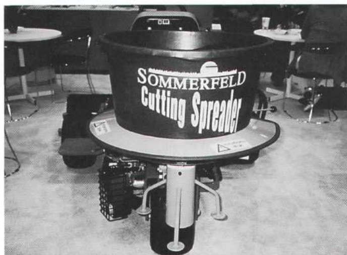
Unique products are everywhere, like this clipping spreader mounted on the back of a triplex greensmower.
