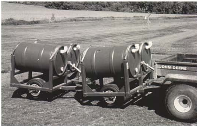
Figure 1. Golf car traffic simulator ready for research at the Noer Facility.
