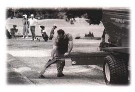
Backfill ditchlines, build cart paths, or place wood chips and compost around trees, plants and in flower beds. The cross conveyor can move in any direction.
