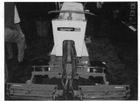
the first triplex greensmower from the late 1960s,
