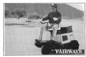
The GA™ 30 Aerator from Ryan can deliver green quality aeration to the entire course. Variable core spacing makes it as good on the fairways as it is on the greens and tees. You can aerate to a depth of 3 3/4" with this single piece of equipment. The 18 h.p. engine produces six m.p.h. speed for fast transport on and off the course.
