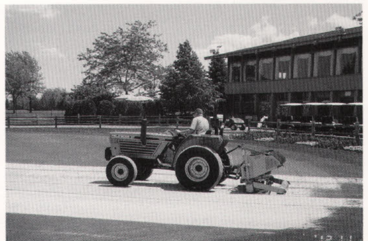
Side view of Dave Strang at work with a Verti-Drain aerifying through sand top dressing with ½" and ¾" solid tines.
