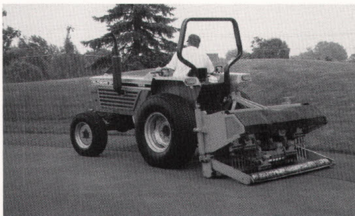
Side view of Dave Strang at work with a Verti-Drain equipped with ½" solid tines.
