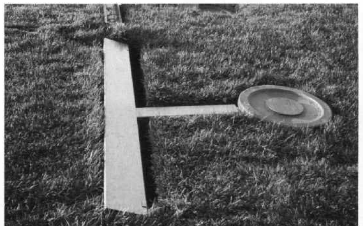
Figure 2. The runoff collection system includes a long rectangular frame which collects the runoff and funnels it into the large trash can on the downside of the slope.
