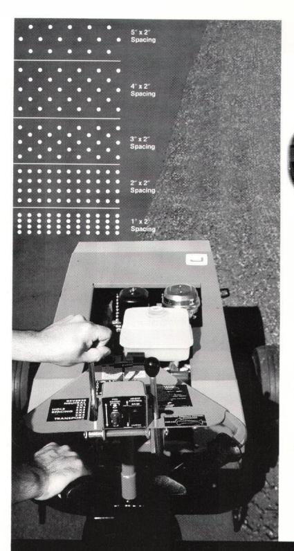
With the two new Jacobsen Aero King aerators, you get the widest selection of hole spacings on the market to handle changing aeration needs quickly and easily. Simply shift gears to select just the right pattern for the job.
