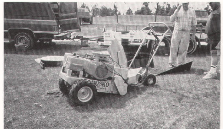
Here's an interesting machine for root pruning trees and installing herbicide barriers.
