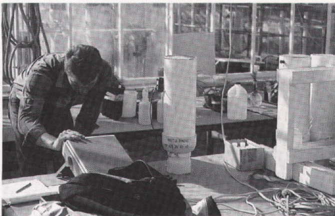
Fig. 1. Jeff measuring soil moisture with the time domain reflectometer.
