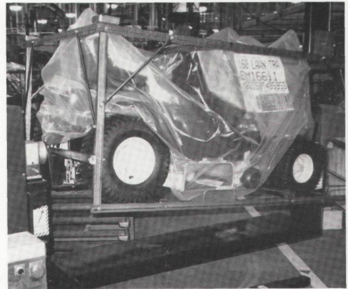
Each vehicle is covered with plastic which is heated for shrink wrapping.
