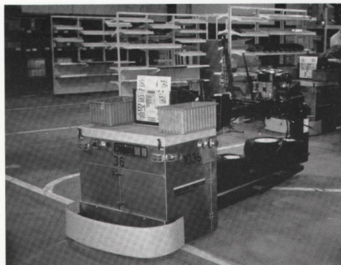
The heart of the focus factory - the AGVL. This one has come from the first island. Note white lines on floor - they mark the path the vehicles follows.
