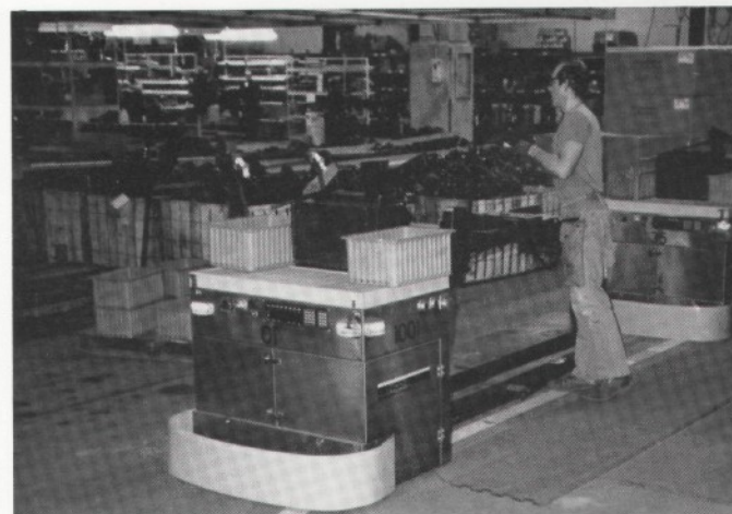
The AGVL robot is readied for a trip through the various assembly islands.
