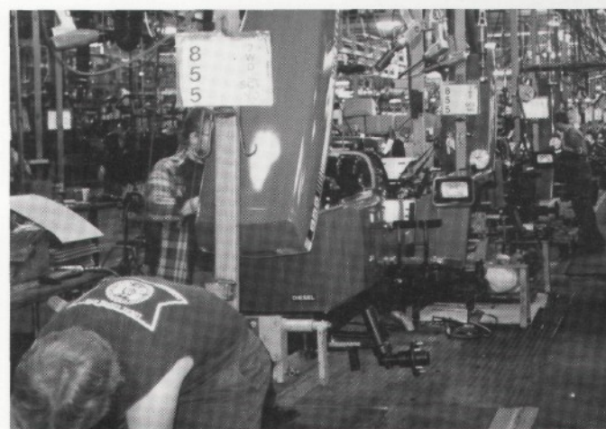
A conventional assemblyline of the John Deere Horicon Works. Here are John Deere 855 tractors under assembly.
