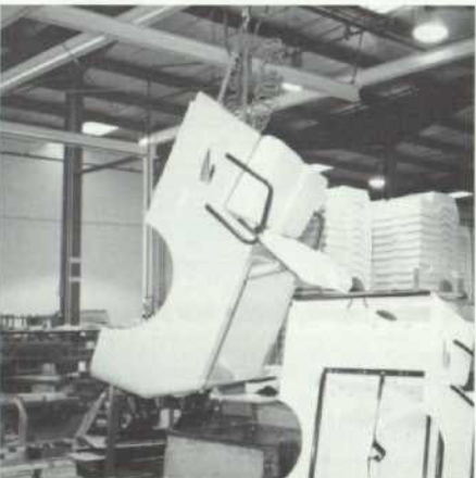
A car body comes from a subassembly area and is married to a chassis on the primary assembly line.
