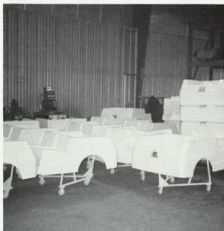
Golf car bodies ready for the paint booth.
