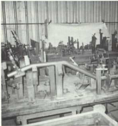
Jigs for frame fabrication.
