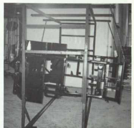
Pieces just out of the paint booth. Parts are cleaned in a phosphate material before they are electrostatically painted.
