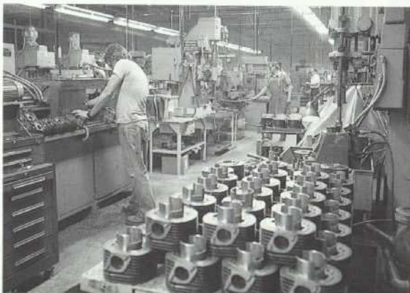
Engine manufacturing by the "cell concept"; one man performs many machining operations.
