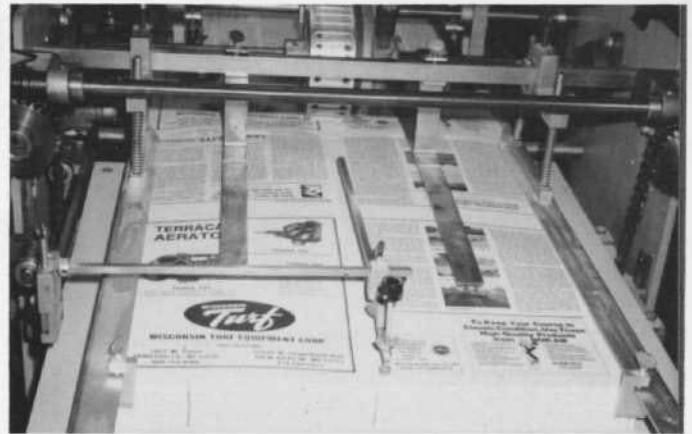
One of the signatures lays ready on the tech-table of the folder.
