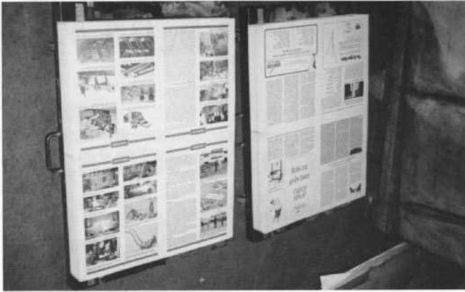
Two of the 8-page signatures for the Grass Roots lay drying after all colors have been "laid down," and are waiting to be folded.
