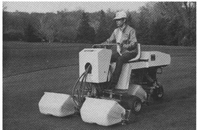
The first all-hydraulic riding triplex greensmower was introduced in 1969—Jacobsen's Greens King.
