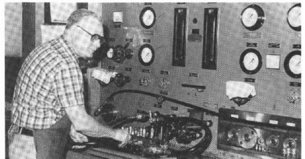
A hydraulic hose pressure testing center checks hydraulic hoses before they are installed in Jacobsen products.
