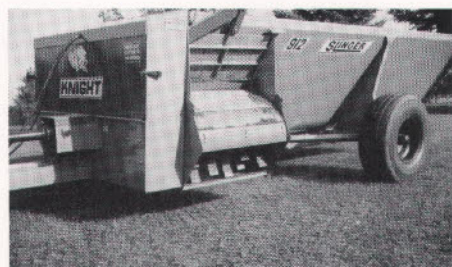
The Knight spreader is an extremely well-built and heavy duty machine. The flail bars you see at the delivery chute each weighs 10 pounds.
