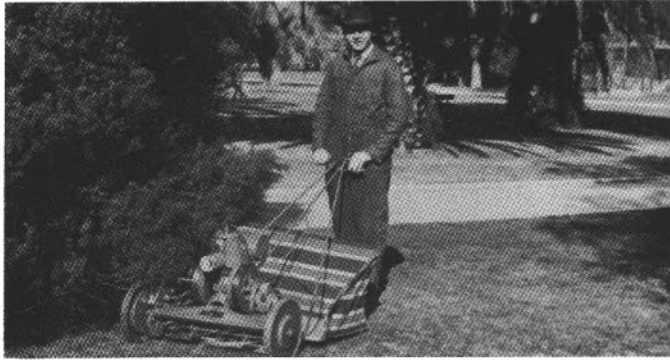
Jacobsen's 4-Acre Mower, introduced in 1921, was the first mower equipped with a gasoline engine specifically tailored to power mower specifications.
