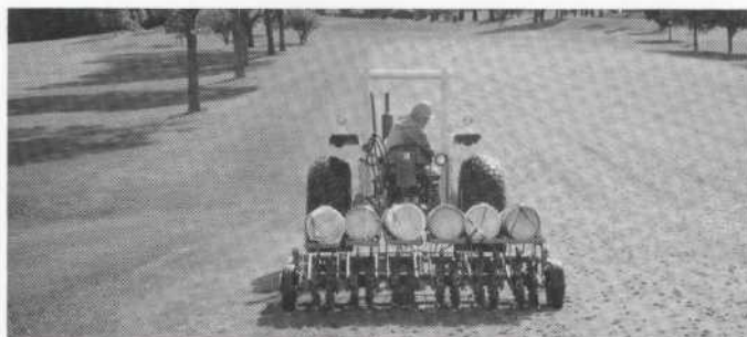
At times the Renovaire does a fairly good job of aerifying, although the number of cores and volume of soil are small.
